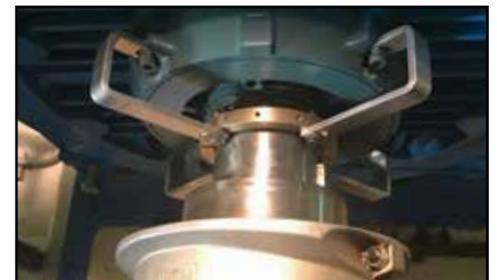
*The Smart CDR can be installed with a variety of mounting configurations, including press-in, clip-on, epoxy, bolt-through, side-mount and flexbracket.*
